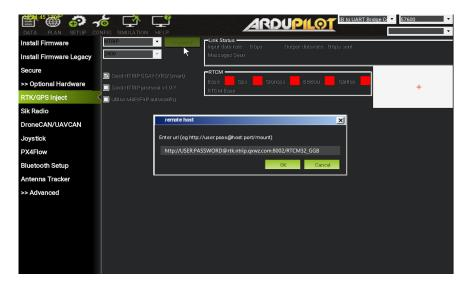
In this format, USER is the username for the FindCM service account applied for by the user, PASSWORD is the corresponding password, rtk.ntrip.qxwz.com is the FindCM service address for the Qianxun positioning server, 8002 is the port broadcasting WGS84 coordinate system data, and RTCM32\_GGB is the data source for broadcasting RTCM 3.2 format data.
