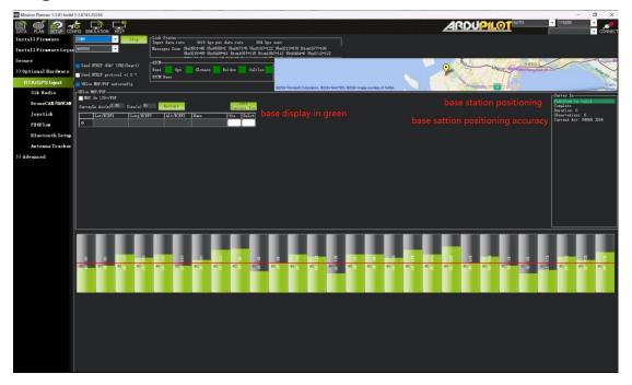
The GPS status will display rtk fixed, indicating that the system has successfully entered RTK positioning mode.
