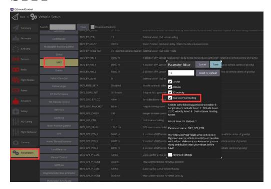
**GPS\_YAW\_OFFSET:** If the primary antenna is located at the front, set the yaw offset to 0. Angles increase in a clockwise direction. If the primary antenna is on the right side of the vehicle and the secondary antenna is on the left side, set the offset to 90 degrees.
