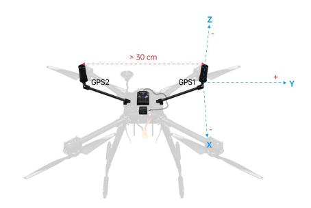
Set the position of the main and secondary antennas for the SIYI RTK Positioning and Orientation Module:
