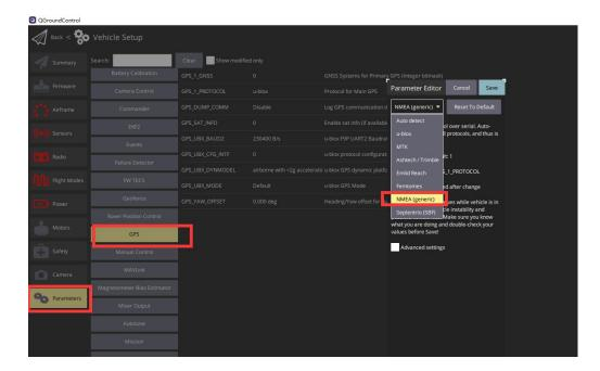
Please note that the above parameters assume you have connected the positioning and orientation module to the GPS MODULE interface. If you are using a different port, you must configure the baud rate and protocol using the respective parameters.
