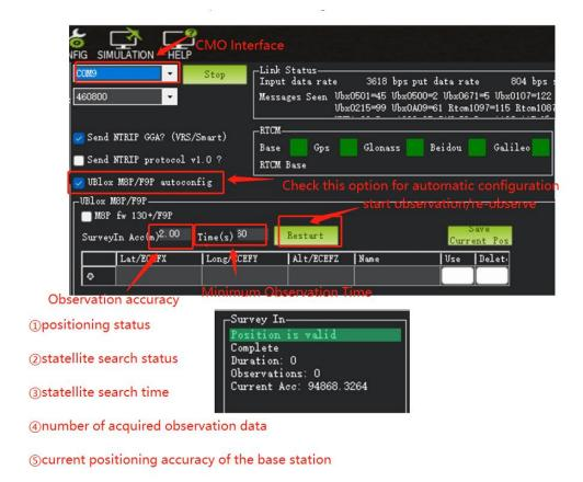
It is recommended to check the option for automatic configuration of the F9P, set the observation accuracy to 2.5, and the minimum observation time to 60s.
