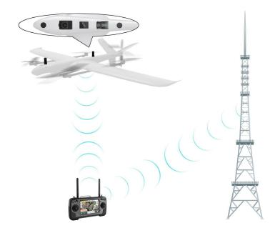
Use the SIYI handheld ground station to run the Mission Planner ground station software, connecting the SIYI handheld ground station to the mobile internet. Go to "Initial Setup > RTK > NTRIP."
