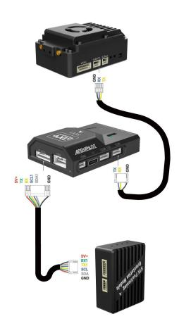
Refer to the diagram above to connect the RTK mobile module to the flight controller, while the flight controller is connected to the airborne data link.
